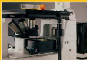
The epi-fluorescence module has the brightest illumination and 4 filter cube capability.
