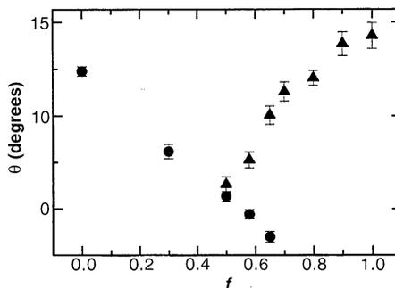
**Fig. 2.** Contact angles ( $\theta$ ) for PS (circles) and PMMA (triangles) on P(S-r-MMA) brushes as a function of  $f$  in the random copolymer. The droplet height  $h$  and diameter  $d = 2r$  were measured for 10 different droplets on each sample, and the contact angle was calculated by assuming a spherical cap shape and using the formula  $\cos \theta = 1 - 2(h/r)^2$ . For a typical droplet,  $h$  was  $\sim 150$  nm,  $r$  was  $\sim 10$   $\mu\text{m}$ , and  $h \ll r$ .
