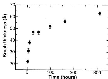
**Fig. 1.** Grafted layer thickness as a function of the annealing time for hydroxyl-terminated polystyrene ( $M_w = 1 \times 10^4$ ) at  $140^\circ\text{C}$ .
