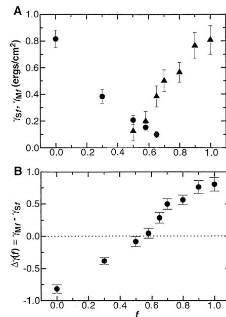
**Fig. 3.** (A) Interfacial energies  $\gamma_{Sr}$  and  $\gamma_{Mr}$  and (B)  $\Delta\gamma(f) = \gamma_{Mr} - \gamma_{Sr}$  for PS (circles) and PMMA (triangles) on a P(S-r-MMA) brush as a function of  $f$ . The near-linear variation of  $\Delta\gamma$  with  $f$  is in keeping with theoretical arguments (26).
