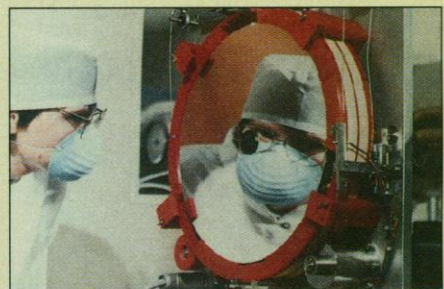
Steady gaze. Hipparcos’s 29-centimeter main mirror looks in two directions at once, allowing it to compare stellar movements in different parts of the sky.
