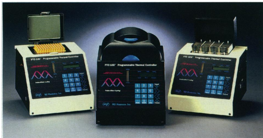
Left to right: A PTC-100-96AgV with a speedy silver-gold block that can ramp at up to 2.5°C/sec, a PTC-100HB with improved Hot Bonnet heated lid that applies heat and pressure to the tops of tubes or plates for oil-free reactions, and a PTC-100-16MS that holds 16 slides & 24x0.2ml tubes for in situ .
