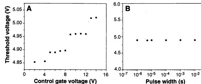
**Fig. 4.** Threshold voltage of the SEMM as a function of (A) the charging voltage on the control gate (voltage pulses of 10 ms), showing a staircase relation with an interval of  $\sim 4$  V, and (B) the charging time while the charging voltage pulse is fixed at 10 V, indicating a self-limited process.
