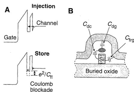
**Fig. 5.** (A) Schematic band diagram before and after injection of an electron into the dot. A single electron stored in the dot can raise its potential by  $e^2/C_{tt}$ , blocking the entry of other electrons from the channel ( $C_{tt}$  is the total capacitance of the floating gate). (B) Schematic cross section of the device showing the capacitive coupling between various elements.
