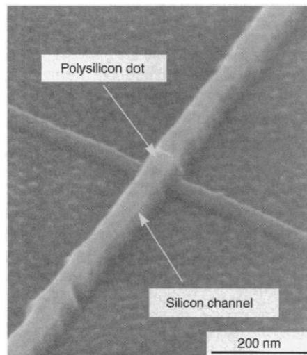
**Fig. 2.** Scanning electron micrograph of the narrow silicon channel with the polysilicon dot on top, before size reduction by thermal oxidation. The width of the channel and the size of the dot are both 50 nm. The lines in the buried oxide, included for easy alignment, come from the second-level EBL and have no effect on device behavior.
