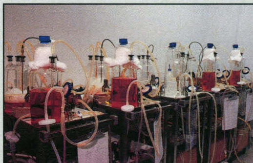
Bioreactor used for large scale production of Eukaryotic cells and cell products. (Fibroblasts, Monoclonals, Chinese hamster ovary, Baculovirus expression, etc.)
