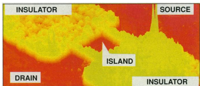
Island-hopping. A vanishingly small island placed in the middle of a device's semiconducting channel compels electrons to hopscotch single file between the source and drain electrodes.
