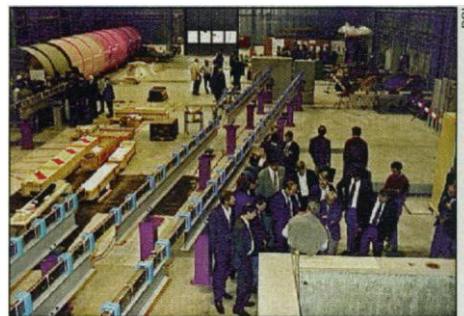
Particle pathways. SINQ's neutron guides direct neutrons from source to instrument.
