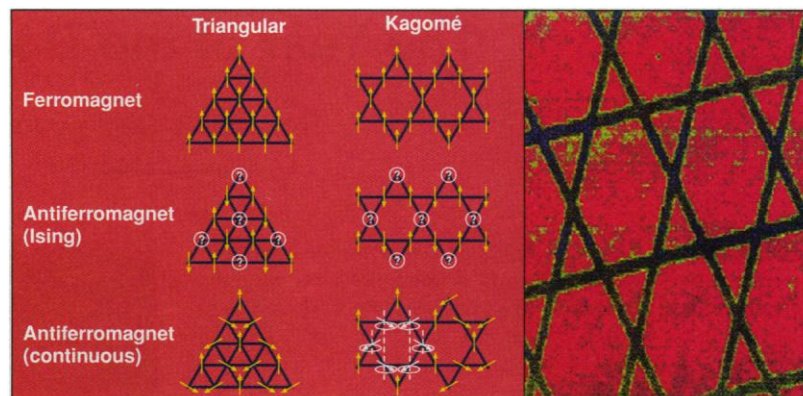
Spin control. (Left) A schematic of the triangular and Kagomé spin systems; the six white continuous spins on the Kagomé lattice can be rotated by 180° without affecting the system. (Right) A micrograph of a Kagomé superconducting network; each side of a hexagon is 2 \mu\text{m} . [Courtesy M. J. Higgins, S. Bhattacharya, P. M. Chaikin, S. Sethuraman, and R. Bojko]
