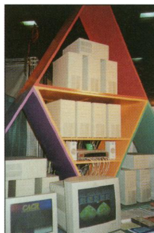
Piling them on. Sixteen Pentium Pro processors, linked by a local area network, make a gigaflops supercomputer, a strategy embodied here in a machine called Hyglac.
