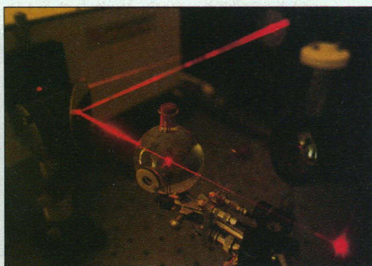
Bubbling mystery. Laser passes through sonoluminescence flask at UCLA. Bubble, seen in another lab, emits light when ultrasound swells and collapses it (below).
