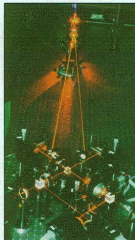
Alice gets the message. In a laser-driven apparatus, the transmitter (Bob) takes advantage of entangled photon states to send one of three different data bits by manipulating a single photon.
