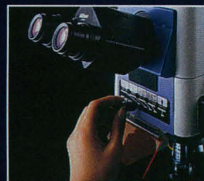
The E800 features a 5-position linear slider, making it faster and easier than ever to change epi-fluorescence filter positions.
