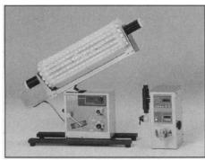
The system consists of 16 locular columns, each consisting of 37 chambers. The rotation speed is adjustable from 0 to 100 rpm with digital readout of the speed. The angle of the columns is adjustable from 0° to 90°. The system is biocompatible, with all wetted parts made of Teflon, polyetherketone, or glass. DyChrom. Circle 139.
