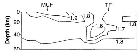
**Fig. 3.** The  $V_p/V_s$  ratio model for the southern Urals. The high values can be interpreted to represent mafic and ultramafic rocks, and the low values, rocks with felsic affinities. The high values at shallow depths coincide with the surface locations of the Kraka massif and the Magnitogorsk volcanic arc, and the low values coincide with the Chebik granitic massif. MUF and TF indicate the surface locations of the Main Uralian and Troisk faults.
