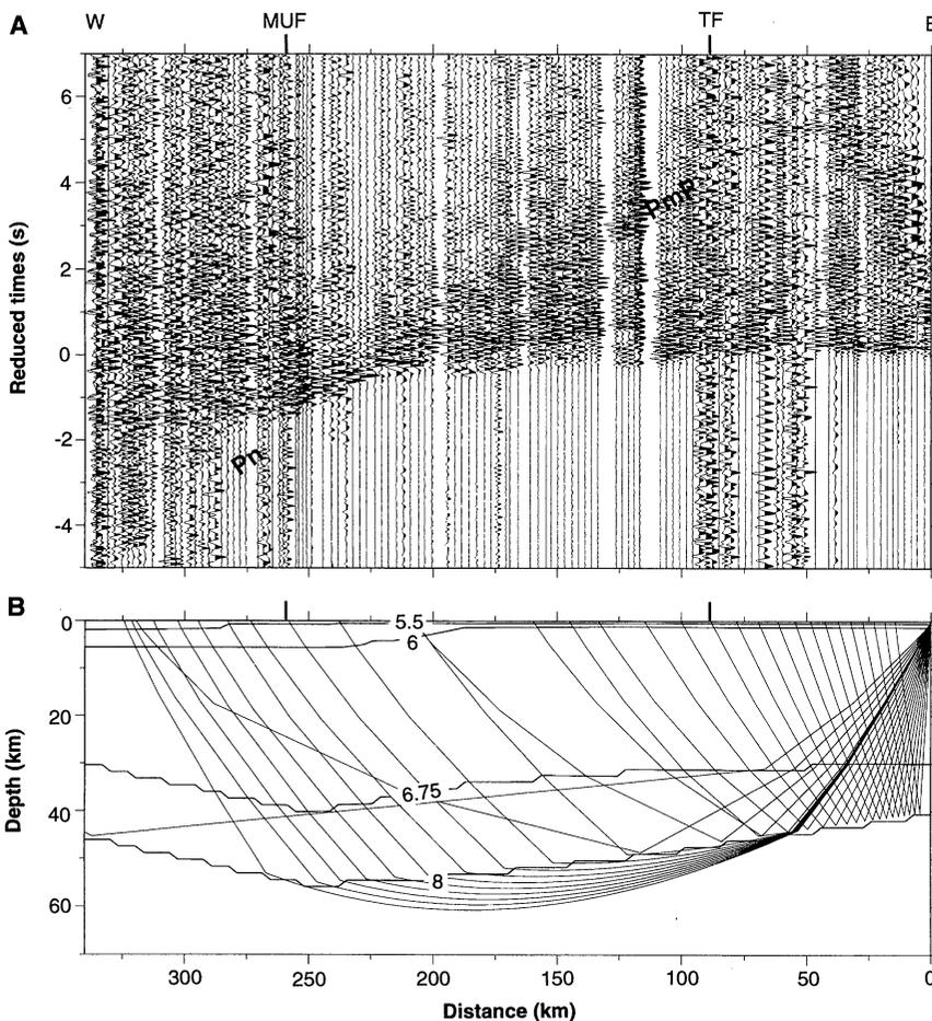
**Fig. 2.** (A) P-wave record section for shot 4. See Fig. 1 for interpreted arrivals. (B) Ray-tracing diagram, illustrating the sampling of the Moho discontinuity for this shot. (The labeling is the same as in Fig. 1.) Distance 0 marks the location of the shot [see S4 in figure 1 of (4)].
