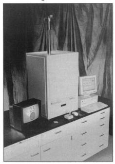
eration region and by reducing matrix background. The instrument is designed to take MALDI-TOF technology out of the research mass spectroscopist's lab and put it in the hands of the protein scientist and molecular biologist working on problems they encounter every day, such as sequencing, glycosylation analysis, and variant determination. PerSeptive Biosystems. Circle 138.
