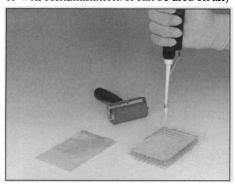
96-well thermal cycler with a heated lid. CycleFoil Plate Sealer and Roller are for sealing PCR products for storage in 96-well arrays. The adhesive-backed aluminum foil, sealed with a firm roll, forms an evaporative barrier. Individual samples can be recovered by piercing the thin foil with a pipette tip while leaving the remaining wells sealed and uncontaminated. Robbins Scientific Corp. Circle 139.
