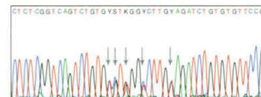
Direct PCR sequencing of the highly polymorphic HLA-B gene using a dye primer kit with the AmpliTaq FS enzyme.
