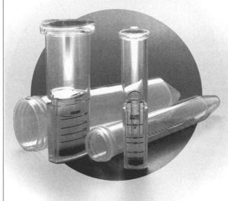
The Ultrafree-®4 Centrifugal Filter Device lets you process more samples in less time by eliminating the need for an inverted spin. Like our Ultrafree-15 unit for processing up to 15 mL of protein, the Ultrafree-4 device incorporates our high-flux Biomax™ (PS) membrane for excellent protein retention and recovery. And, the vertical design makes recovery easy, without spinning to dryness. Just pipet the sample from the concentrate pocket after a single spin.
