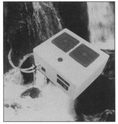
often difficult. This device obviates the need to schedule experiments around the availability of a lab sink and to monopolize the sink for the duration of the experiment. The device is fitted with a pump, a heat exchange coil, and two fans to dissipate the heat
