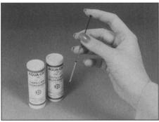
when pressed down by a reusable plunger. The design prevents a second use, eliminating the possibility of cross-contamination. They are available in sizes from 10 to  $100 \,\mu$ l. Drummond Scientific. Circle 139.
