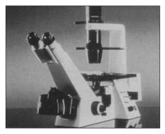
a stage height of only 190 mm and working distances between 53 mm and 190 mm, it is suited for cell culture vessels of all kinds. The sliding condenser offers brightfield scanning illumination with maximum working distance for observing roller bottles and other large flasks. Carl Zeiss. Circle 139.
