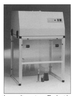
lates or earlier experiments. The ultraviolet lighting inactivates DNA and RNA contamination within minutes to ensure reliable results during sample preparation for nucleic acid amplification. Sample protection is provided to better than class 100 by bathing the work surface with 0.12  $\mu m$  of filtered air. The VLF24 provides true laminar air flow and ensures nonturbulent air
