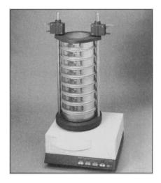
results with much less noise than conventional "rotating and tapping" instruments. The Basic Siever includes an analog timer and amplitude control. The AS200 Digit Siever features a digital timer and analog amplitude control. The AS200 Control Siever features a digital timer, digital control of interval duration, and digital amplitude control. **Brinkmann Instruments. Circle 142.**
