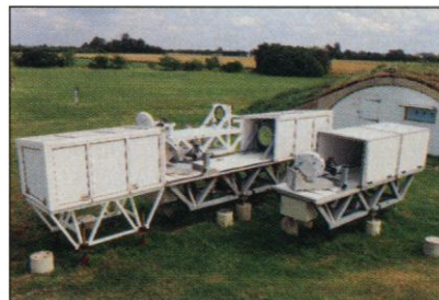
All together now. COAST's four mirrors send light to a buried optics laboratory, where it is merged and analyzed.
