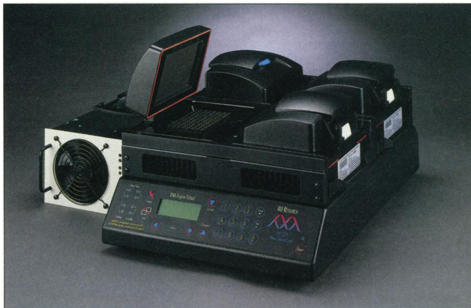
The PTC-225 Tetrad™ with four independent blocks, each with its own Hot Bonnet™ heated lid.
