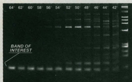
Optimization of PCR primer annealing temperature with the RoboCycler ® Gradient 96 system*
