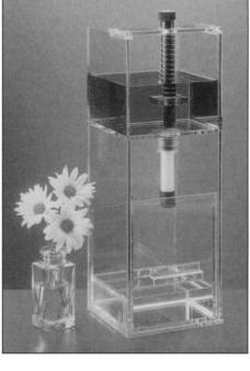
demonstrate binding of stain. Once buffer is passed through the resin, it is safe for disposal down the drain, which can save significantly in hazardous waste expenses. The laboratory size unit can process more than 200 liters of buffer and bind in excess of 100 mg of stain. American Bioanalytical. Circle 145.
