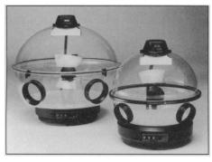
eliminate contamination by both microorganisms and DNA. Clean room conditions can be achieved in approximately 5 min. The chambers provide audio as well as visual indication that they are ready for use. DNA contamination is eliminated by ultraviolet irradiation at 254 nm for 40 min. Safetech. Circle 137.
