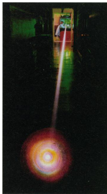
Long light. Optical channel formed as an intense laser pulse propagates down a laboratory hallway. [Photo courtesy of G. Mourou, University of Michigan.]
