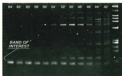
Optimization of PCR primer annealing temperature with the RoboCycler ® Gradient 96 system*
