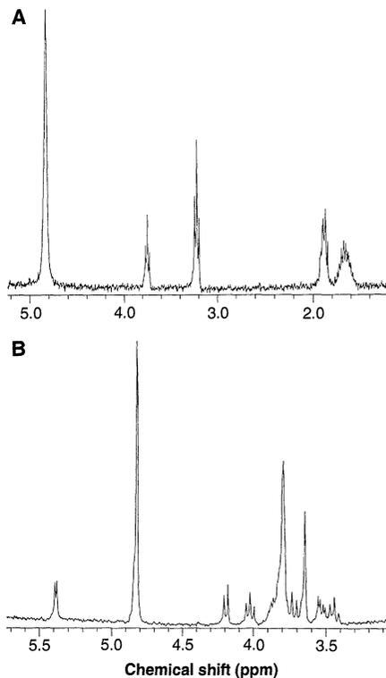
**Fig. 6.** (A) Arginine-HCl and (B) sucrose microcoil NMR spectra. The data acquisition time was 1 min and line broadening was used. The arginine spectrum has 0.53  $\mu$ g (2.5 nmol) of sample in the 5-nl capillary detection cell. The sucrose spectrum has 0.86  $\mu$ g (2.5 nmol) of sample in the cell. The LODs appear in Table 1, and data acquisition parameters are in (13).
