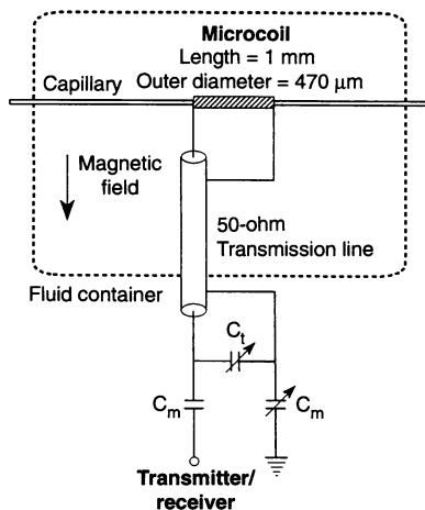
**Fig. 1.** Layout and circuit for microcoil NMR (7);  $C_1$  and  $C_m$  are the tuning and matching capacitors, respectively.
