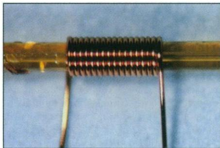
**Fig. 2.** Typical microcoil and polyimide-coated, fused-silica capillary. The coil is composed of 50- $\mu\text{m}$ -diameter copper wire, has a length of 1 mm, and an OD of 470  $\mu\text{m}$ .
