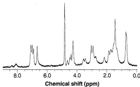
**Fig. 7.** A 300-MHz microcoil NMR spectrum of *Aplysia californica*  $\alpha$ -bag cell peptide (residues 1-7). The 5-nl detection cell contains 3.0  $\mu$ g (3.3 nmol) of peptide. The LOD is 112 ng (124 pmol). Data acquisition parameters are as in (13).
