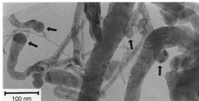
**Fig. 4.** A TEM image of polycrystalline InP fibers obtained from reaction 1a (PhSH catalyst, refluxing toluene solution). The arrows point to the In flux particles (frozen droplets) at the fiber tips.
