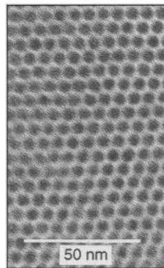
**Nano order.** Transmission electron micrograph of a face-centered cubic array of dots, each 48 Å in diameter [adapted from (1)].
