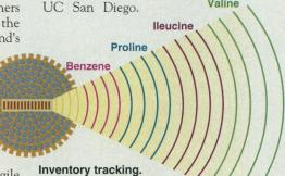
A radio-emitting microchip can encode the identity of molecules grown on surrounding beads.
