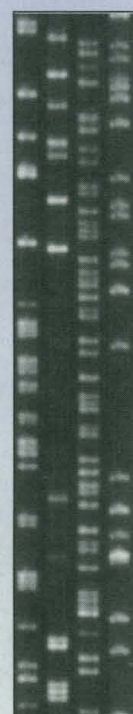
M13mp18 plasmid was sequenced using the SequiTherm Long-Read Kit and LI-COR® Model 4000L Sequencer; reads of 800 bases or greater at >99% accuracy are possible. (Results courtesy of S.L. Sutter, LI-COR, Inc.)
