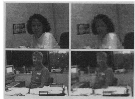
Fig. 3. Two panchromatic 192 pixel by 256 pixel test images (left) compressed and decompressed (right) by a partially trained replicator network. Images are first divided into disjoint 64-pixel by 64-pixel tiles. The 4096 eight-bit pixel brightnesses of each tile make up its \mathbf{x} vector. These \mathbf{x} 's are used to train or test the replicator network (the images shown were not used during training). The network used had m = 4096 , n = 40 , N = 256 , and L_2 = L_4 = 410 (compression ratio = 102.4:1). After reconstruction, the boundaries between the tiles were deemphasized by a smoothing operation. This replicator network has 3,396,476 weights.
