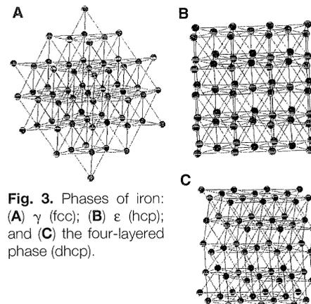
**Fig. 3.** Phases of iron: (A)  $\gamma$  (fcc); (B)  $\epsilon$  (hcp); and (C) the four-layered phase (dhcp).
