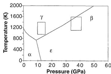
**Fig. 1.** Part of the iron phase diagram showing the pressure-temperature fields of our study. On laser heating, iron at lower pressures was largely converted to the fcc phase. Temperatures shown are approximate. At high pressures, the iron shows a distinct phase transformation from hcp to possibly a dhcp form of iron. According to Saxena *et al.* (2, 4),  $\beta$  iron would be stable at 1400 K between 35 and 40 GPa. The  $\delta$  phase is not shown.
