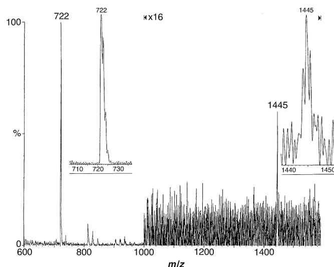
**Fig. 1.** Electrospray MS (+) spectrum of a 0.02 to 0.05 mM solution of  $(\text{C}_{59}\text{N})_2$  in toluene. The insets are expansions around the 722 and 1445  $m/z$  peaks. The expanded patterns give an excellent fit to the calculated isotope mass ratios.
