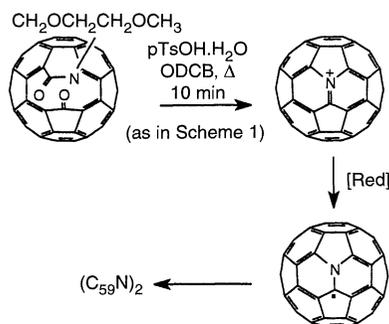
**Scheme 2.** Proposed cascade of events in the pTsOH.H<sub>2</sub>O-initiated formation of (C<sub>59</sub>N)<sub>2</sub> from N-MEM ketolactam **1** in refluxing ODCB.
