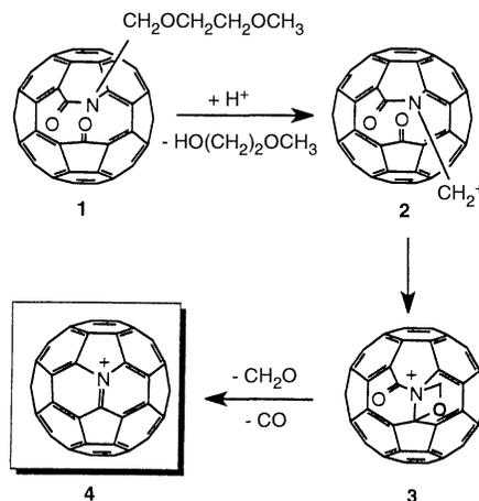
**Scheme 1.** Proposed mechanism for the gas-phase formation of azafulleranium  $C_{59}N^+$  (4) from N-MEM ketolactam 1 in FABMS.
