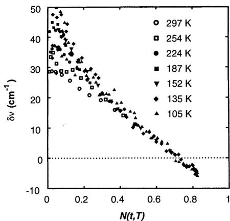
**Fig. 3.** Average spectral frequency shift  $\delta\nu(t, T)$  of photolyzed molecules versus  $N(t, T)$ . Data from all values of  $T$  fall on essentially the same curve, which implies that spectral shifts during ligand recombination result from kinetic hole burning, rather than from conformational relaxation. The deviation for  $T > 250$  K (at  $N < 0.2$ ) can be attributed to population of the additional geminate state C.
