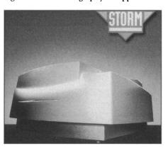
that require the use of radioisotopes. The optical components required for the system's three-in-one capability are integrated into a single scanning element. The system's 35 cm by 43 cm scanning area accommodates sequencing gels and other large samples. Molecular Dynamics. Circle 141.
