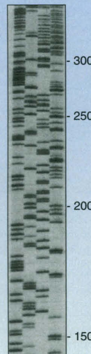
C. elegans M13 subclone sequenced using the SequiTherm Long-Read™ Kit and an ABI Model 373A "Stretch" Sequencer. Trace data show excellent peak resolution 700 bases from the primer. (Results courtesy of L.A. Weinstock & E.R. Mardis, Wash. Univ. Genome Sequencing Center)
