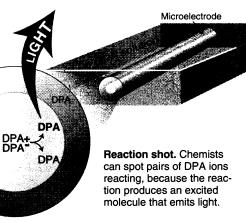
ing DPA molecules in an organic solvent and then rapidly reversing a potential in an electrode to first create a burst of positive ions followed by another of negative ions in the solution. The electrode had to be extremely small, a mere 10 microns in diameter. A device this small ionizes far fewer DPA molecules than would a larger variety, reducing the likelihood of overlapping photon bursts that would make it hard to discern the finishing times of the reactions.
