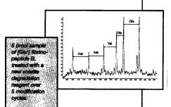
mass accuracy for the LASERMAT™ has been confirmed on real samples as ±0.4Da. Such high precision allows unambiguous identification of all 20 common amino acids. With sample loads as low as 50fmol, the presence of residual buffer salts and excess reagent had no observable suppressive effect on the data.
