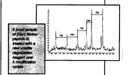
The mass accuracy for the LASERMAT<sup>TM</sup> has been confirmed on real samples as  $\pm 0.4Da$ . Such high precision allows unambiguous identification of all 20 common amino acids. With sample loads as low as 50fmol, the presence of residual buffer salts and excess reagent had no observable suppressive effect on the data.
