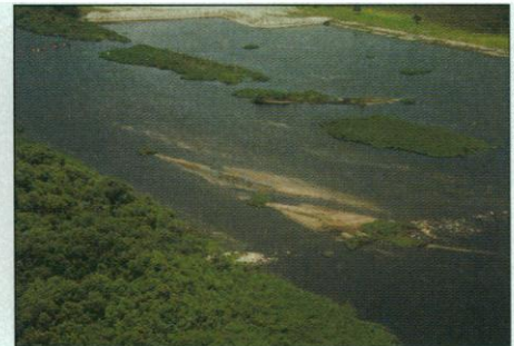
River test bed. Last year, as part of the Kissimmee River test restoration, high embankments were lowered ( left ). By last month, the area (shown at right from a different angle) had been transformed back into a flood plain, and patches of wetland vegetation began to recolonize it.
