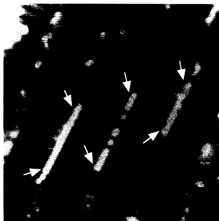
Fig. 5. An STM image (150 Å by 150 Å, V_s = -1.4 V, I = 0.1 nA) showing a pattern of 30 Å pitch lines of dangling bonds written with V_s = +3 V, I = 4.5 nA, and Q = 6 \times 10^{-4} C/cm. The arrows point to sites at which both H atoms of an Si dimer have been desorbed.
