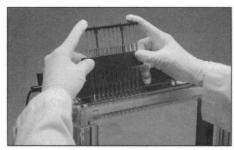
nel pipette for easy transfer of samples from a microwell plate directly to the polyacrylamide sequencing gel. Manufactured from a nonbrittle polyester base material, the combs have exceptional consistency in thickness, temperature stability, and resiliency. Owl Scientific. Circle 138.
