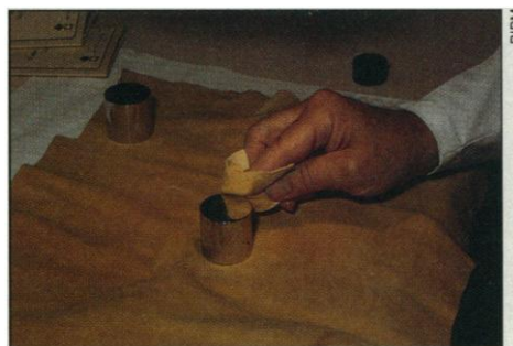
That special touch. Georges Girard uses a chamois cloth to polish contamination from the surface of a standard kilogram replica.
