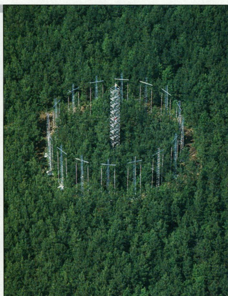
Pumped up. The towers are used to pump CO 2 into Duke's experimental forest plot.
