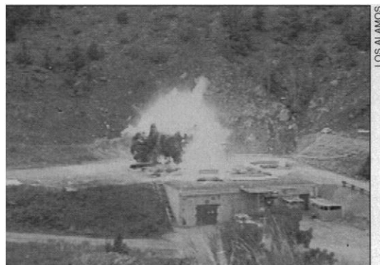
Explosive charge. One of a series of Los Alamos-Arzamas experiments on explosively driven pulsed power.
