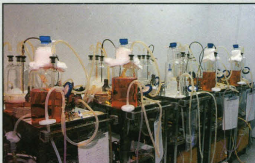
Bioreactor used for large scale production of Eukaryotic cells and cell products. (Fibroblasts, Monoclonals, Chinese hamster ovary, Bacula virus expression, etc.)
